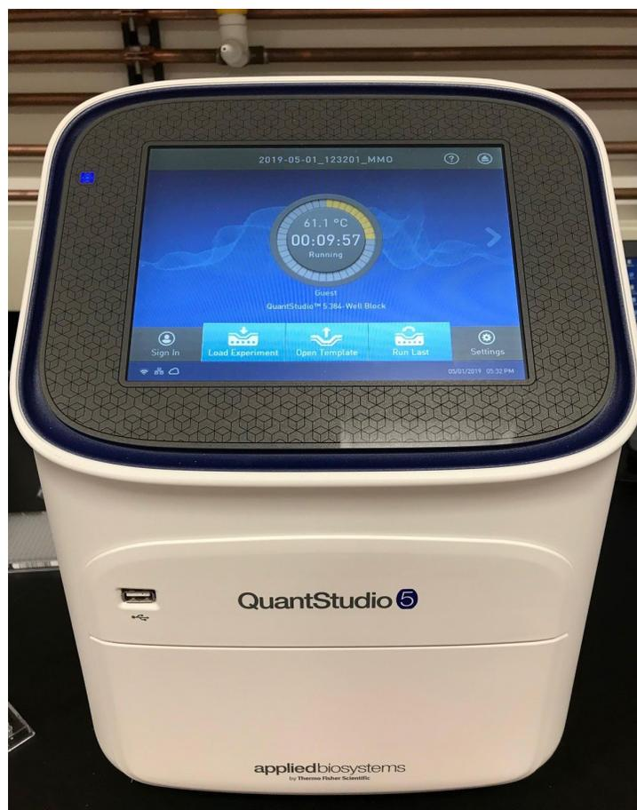
**Figure 2:** QuantStudio™ 5 System (Appliedbiosystems). Samples in a 384-well plate were run by the following fast-mode cycling program (repeated 40 times) for RT-qPCR analysis:  $50.0^{\circ}\text{C}$  for 2 minutes,  $95.0^{\circ}\text{C}$  for 20 seconds,  $95.0^{\circ}\text{C}$  for 1 second, and  $60.0^{\circ}\text{C}$  for 20 seconds.
