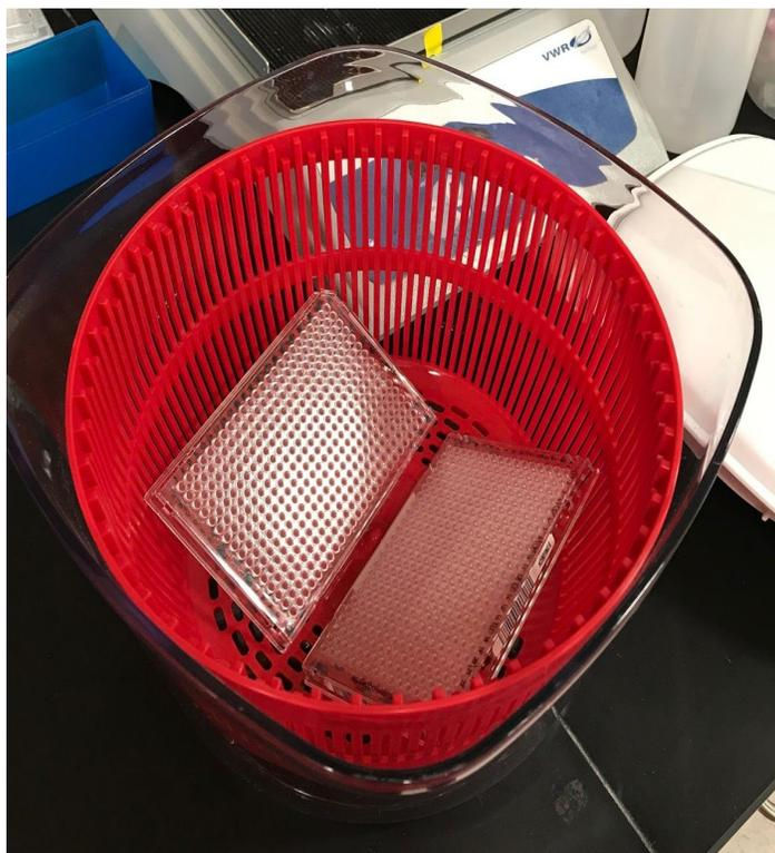
**Figure 1:** Spinning apparatus for 384-well plate (with balance) prior to RT-qPCR. Sample wells frequently contained bubbles after pipetting; spinning was necessary to eliminate bubbles, as RT-qPCR is affected by bubble presence.
